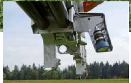
Distance Control: Ultraschallsensor
