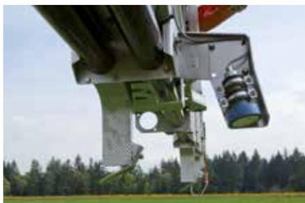
Distance Control: Ultraschallsensor
